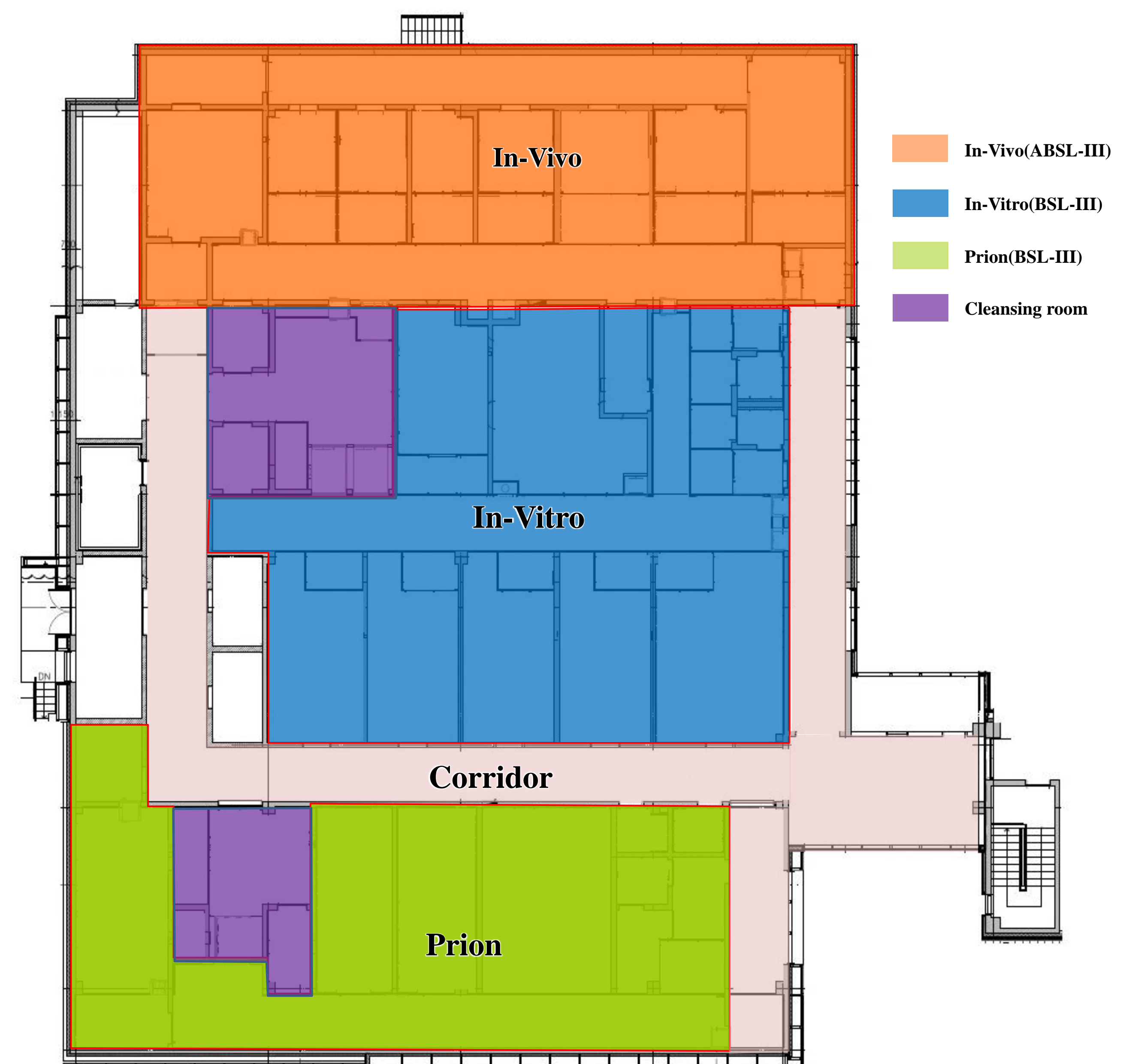
Figure. 1 Layout of a new BSL/ABSL-III facility
